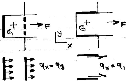
Both joints are subjected to primary (force) loading only - there is no centrifical moment or secondary intensity i.e.  $q = [q_x \ 0 \ 0]$ ,  $q_x = F/L$ . The difference between the joints, for same  $F, L$  is that  $q_x$  is a  $q_3$  (or  $q_2$ )
