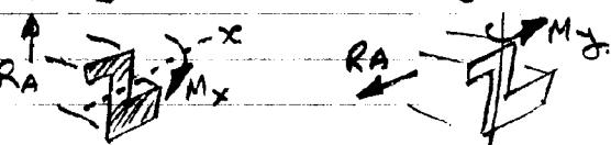
$$M_{Bx} = -50E6 \text{ N-mm} \quad M_{By} = -15E6 \text{ N-mm} \\ M_{Cx} = -25E6 \text{ N-mm} \quad M_{Cy} = -20E6 \text{ N-mm}$$
